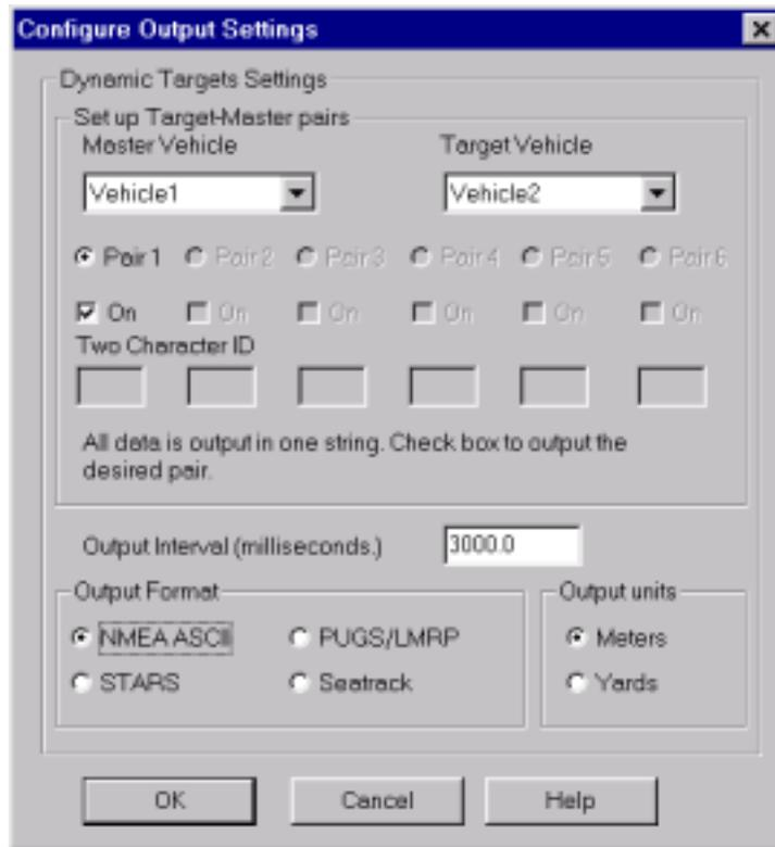
The above dialog allows you to select the required data format and units, as well as which vehicles are to be used to determine the range and bearing between.
